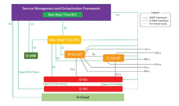
Al Interface between Non-RT RIC and Near-RT RIC to enable policy-driven guidance of Near-RT RIC applications/functions, and support AI/ML workflow - OI Interface connecting the SMO to the Near-RT RIC - O2 Interface between the SMO and the O-Cloud - E2 Interface connecting the Near-RT RIC or more O-CU-CPs/UPs/DUs/O-eNBs - Open Fronthaul CUS-Plane Interface between O-RU and O-DU - Open Fronthaul M-Plane Interface between O-RU and O-DU and between O-RU and SMO.
